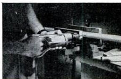
Power drills may be used or conventional wood expansion bits are very effective for boring holes in sheet. Regular auger bits work equally well.
